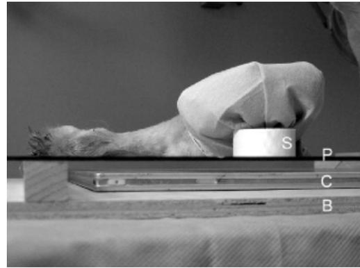
**Fig 2.** Side view of the positioning device. The specimen is placed on the glass plate (P). The dissected thigh muscles and the proximal femur are wrapped in cloth. Note the spacer (S) between the glass plate and the trochanter replacing the dissected muscles. The radiographic cassette (C) is resting on the wooden base (B) below the glass plate (P).
