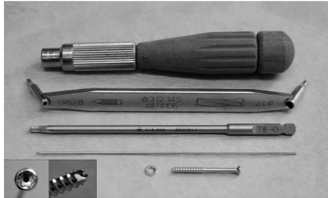
**Fig. 2** Instrumentation set for Ø 2.4 mm cannulated screws: handle with quick coupling, 1.7 mm/0.8 mm double drill guide, cannulated screwdriver shaft Stardrive® T8, guide wire Ø 0.8 mm /length 100 mm, stainless steel washer and 26 mm long cannulated screw Ø 2.4 mm. Magnification: cannulated Stardrive® T8 head, cannulated self-drilling and self-tapping tip.
